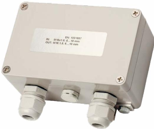
KL termination boxes complete pressure transmitters with hydrometric cables and Pt100 resistance thermometers. Through a special filter in the housing of the box atmospheric pressure reaches the cable's capillary tube.
